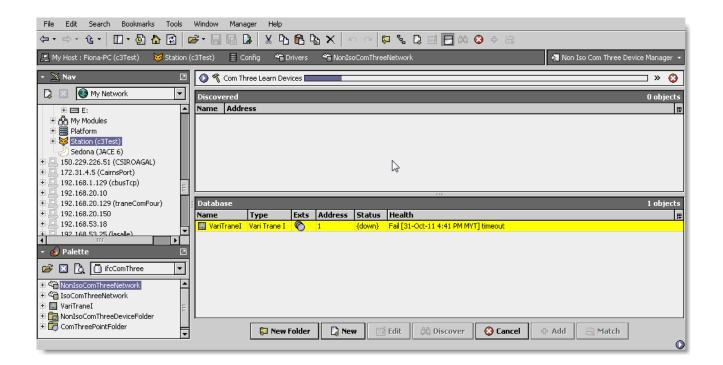
Single or multiple VariTrane devices can be added as device by selecting the discovered row(s) in the top pane, and clicking add. Doing so will cause the "Add" dialog box to appear: Once the device(s) are satisfactorily edited, click "OK" to create the device corresponding to the device property.
